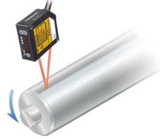
Measuring the eccentricity of a metal shaft
