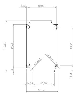
Dashed line shows outline of the mounting boss under PCB board Recommended mounting holes diameter  $\emptyset 3,5 \text{mm}$
