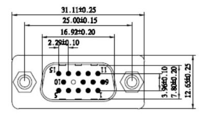
INSULATOR: PBT Glass fibre reinforced UL 94 VO
