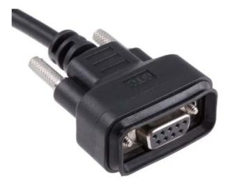
The RS PRO series of waterproof D-sub connectors are a range of ruggedised IP67 connectors designed to be used outdoors or in harsher industrial environments. Designed to fit panel cut outs of 40.0mm the waterproof D-sub series also comes with rear potting on the panel mount connectors. This ensures your panel is still sealed to an IP67 rating even when the connector is unmated. The Push-Fit with dual Screws mating allows for a secure connection. **Features & Benefits:**
