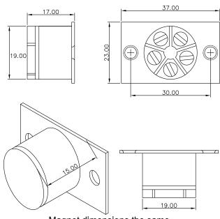
Magnet dimensions the same as switch dimensions except depth 15mm
