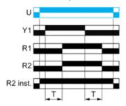
Function Act: On-Delay & Off-Delay with Control Signal & With Pause / Summation Control
