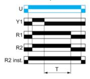
Function Ct: Off-Delay Relay with Control Signal & With Pause / Summation Control
