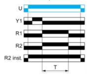
Function Wt: Interval Relay with Control Signal Off & with Pause / Summation Control
