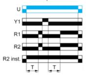
Function C: Off-Delay Relay with Control Signal
