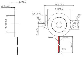
Dimensions : Millimetres Tolerance: ±0.2mm
