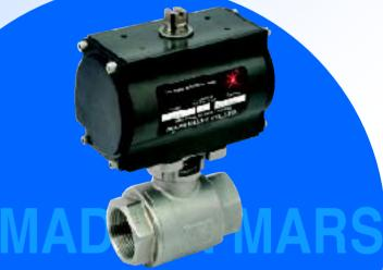
No bracket and adapter are required, the valve stem is an integral part of the actuator drive. The direct valve stem coupling to actuator shaft ensures correct alignment of the valve to the actuator, minimizes stem side loading and backlash during operation, increased service life and performance.
