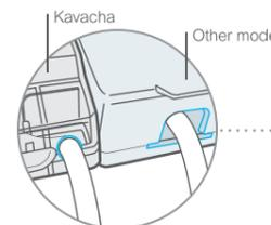
Water and moisture can be completely kept out of the socket cover at all times even with a plug present, since the cover snugly clicks shut around the plug cord, leaving no gap around the plug cord
