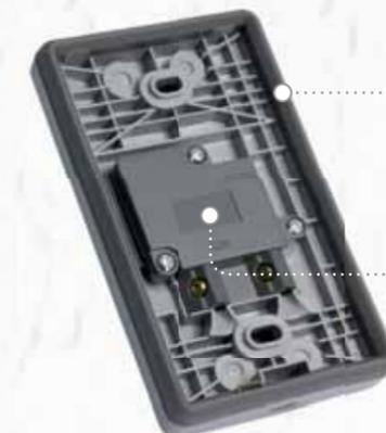
○ Co-injection moulded gasket on the base plate seals tight with the cover plate, avoiding any penetration of water and is more durable than the conventional O-ring design
