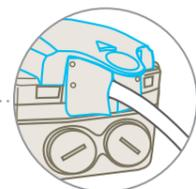
Protection shield for socket outlet to ensure plug is completely kept out of water and moisture at all times, since the cover can be closed snugly and leaves no gap around the plug cord
