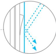
UV-impervious membrane filters out UV and protects the switch from damage caused by sunlight
