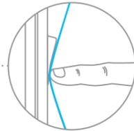
Flexible and durable membrane allows switch to be pressed easily when cover is tightly closed
