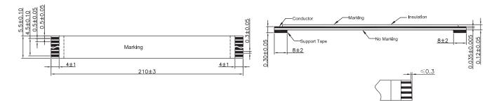
Dimensions: Millimetres Tolerances: ±0.3mm
