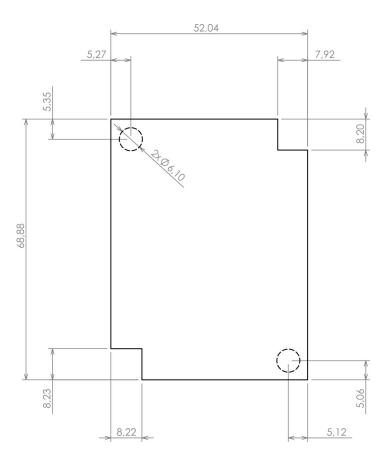
Dashed line shows outline of the mounting boss under PCB board Recommended mounting holes diameter ø3,5mm All dimensions are given within +/-0,5mm tolerance
