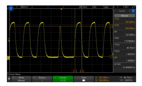
Figure 45 Measuring pulse width with cursors
