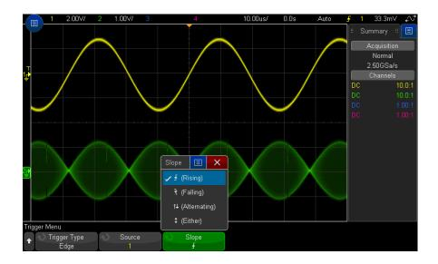
Using Autoscale to Set Up Edge Triggers The easiest way to set up an Edge trigger on a waveform is to use Autoscale. Simply press the [Auto Scale] key and the oscilloscope will attempt to trigger on the waveform using a simple Edge trigger type. See "Use Autoscale" on page 35.
