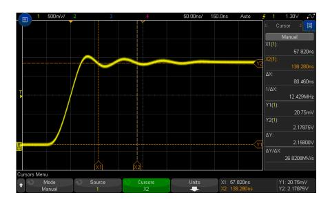
Figure 43 Cursors measure frequency of pulse ringing
