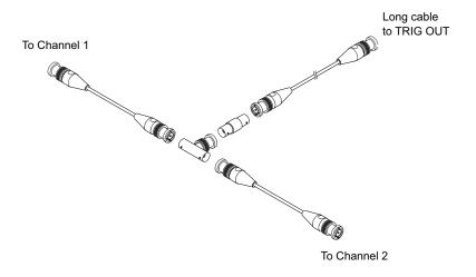
Figure 51 User Calibration cable for 2-channel oscilloscope
