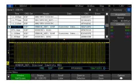
In addition to the standard Time column, the USB PD Lister contains these columns:
