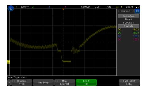
Figure 29 Example: Triggering on Line 136
