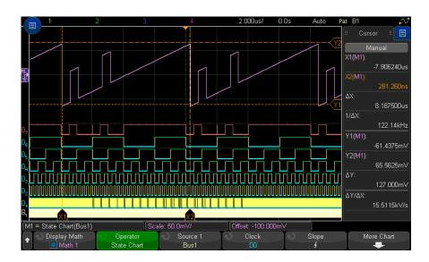
Figure 20 Example of Chart Logic Bus State
