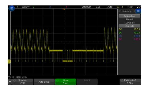
Figure 31 Triggering on Field 1
