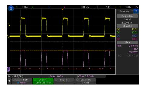
Figure 16 Example of Low Pass Filter
