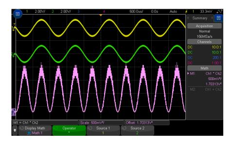
Figure 7 Example of Multiply Channel 1 by Channel 2
