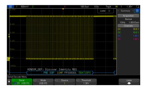
The USB PD decode is displayed as a single bus, with one decode line positioned at the bottom of the waveform area, time-aligned with the associated physical signal. Above the decode line is abbreviated symbolic decode information, shown in white, that describes the header's port power role (bit 8), port data role (bit 5), and message type (bits 4-0).
