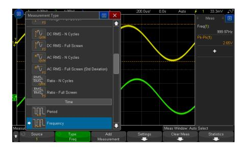
You can also use the touchscreen to select measurements. You can touch the "+" in the Measurements sidebar dialog to open the measurement type menu. See also "Touch Softkeys and Menus On the Screen" on page 53.
