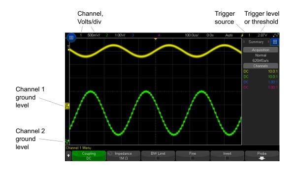
The ground level of the signal for each displayed analog channel is identified by the position of the  $\Rightarrow$  icon at the far-left side of the display.
