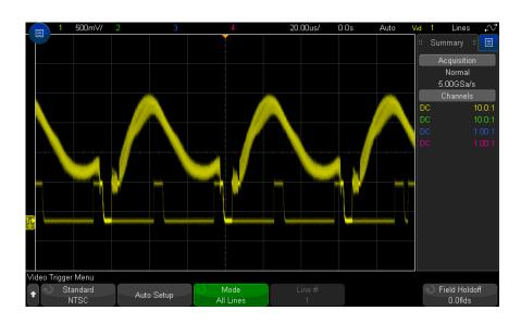
Figure 30 Triggering on All Lines
