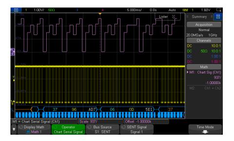
Figure 21 Example of Chart Serial Signal
