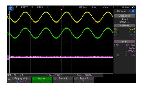
Figure 6 Example of Subtract Channel 2 from Channel 1
