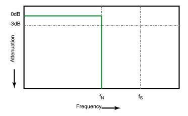
Figure 36 Theoretical Brick-Wall Frequency Response
