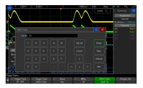
The data value is left-justified in the frame when setting up the trigger. If the base is Hex, the first digit represents the first 4 bits after the start of frame, continuing with the remaining digits in the data value.
