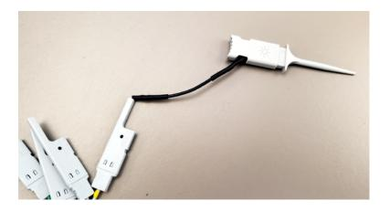
**5** Connect the grabber to a node in the circuit you want to test.
