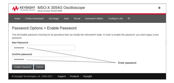
When a password is enabled for the web interface, **Log out** or **Log in** appears in the upper-right corner next to the gear icon.
