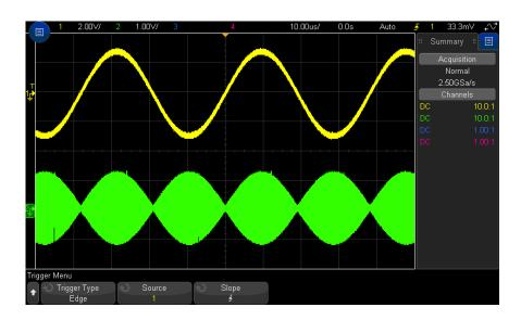
Figure 27 Amplitude Modulation Shown at 100% Intensity
