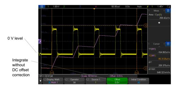
Figure 9 Integrate Without Signal Offset
