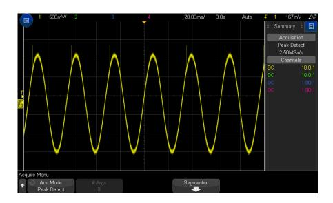
Figure 39 Sine With Glitch, Peak Detect Mode
