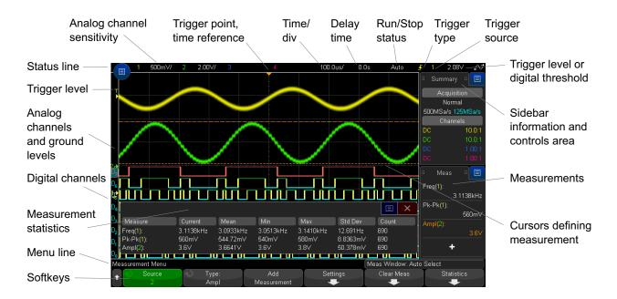
Figure 1 Interpreting the oscilloscope display
