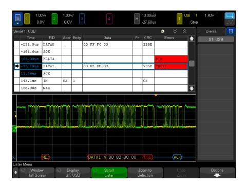
In addition to the standard Time column, the USB 2.0 Lister contains these columns:
