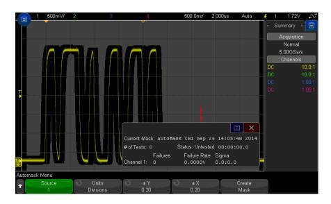
**9** To clear the mask and switch off mask testing, press the Back/Up key to return to the Mask Test Menu, then press the **Clear Mask** softkey.
