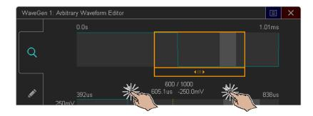
To adjust the value of a point, drag the voltage level handle up or down:
