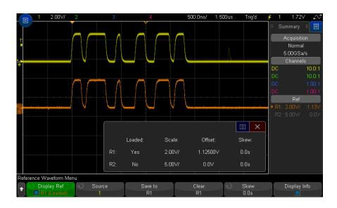
One reference waveform can be displayed at a time.
