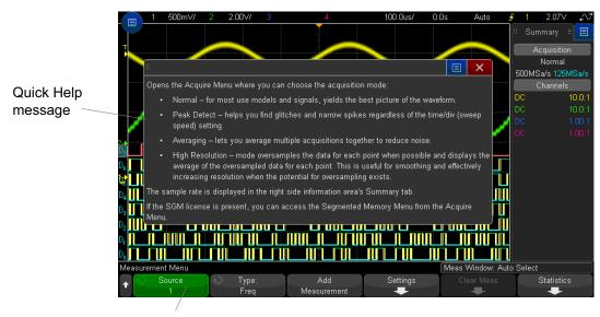
Press and hold front panel key or softkey (or right-click softkey when using web browser remote front panel).
