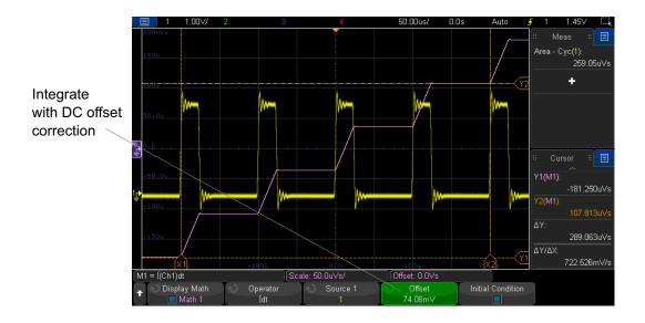
Figure 10 Integrate With Signal Offset
