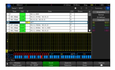
Each Fast or Slow Channel message is represented on its own row. The start time of Slow Channel messages determines their order relative to the Fast Channel messages. Therefore, a Slow Channel message appears before most of the Fast Channel messages that it was built from. This is due to the "Time" column holding the start time of a packet.
