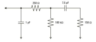
Figure 24 High-Frequency Probe Equivalent Circuit
