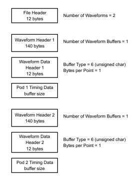
Segmented Memory Acquisition on One Analog Channel The following picture shows a binary file of a segmented memory acquisition on one analog channel.
