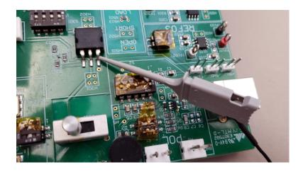
**6** For high-speed signals, connect a ground lead to the probe lead, connect a grabber to the ground lead, and attach the grabber to ground in the device under test.
