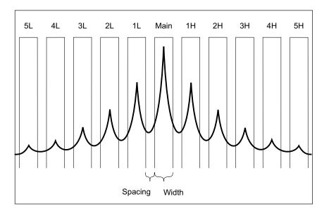
The sideband used for the measurement is selected with the Channel Select parameter. You can select the first through fifth sidebands above or below the main range (1H through 5H above and 1L through 5L below). The full sideband must be in the graticule to be measured. Otherwise, the measurement results will be "Incomplete".
