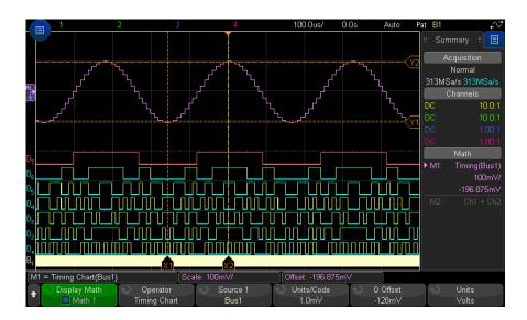
Figure 19 Example of Chart Logic Bus Timing
