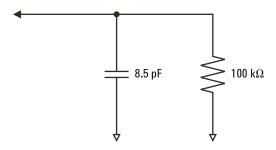
Figure 23 DC and Low-Frequency Probe Equivalent Circuit
