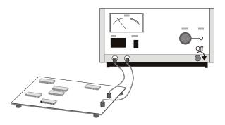
2 Connect the digital probe cable to the DIGITAL Dn - D0 connector on the mixed-signal oscilloscope. The digital probe cable is keyed so you can connect it only one way. You do not need to power-off the oscilloscope.
