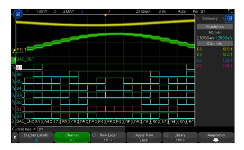
3 To turn the labels off, press the **Display Labels** softkey again.
