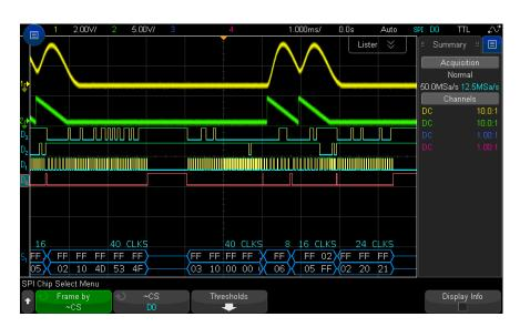
**8** Press the **CS** softkey to open the SPI Chip Select Menu.
