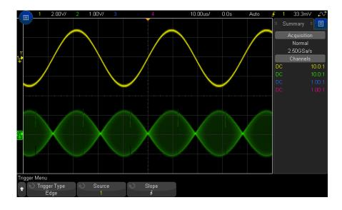
Figure 28 Amplitude Modulation Shown at 40% Intensity
