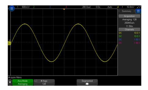
Figure 41 128 Averages used to reduce random noise
