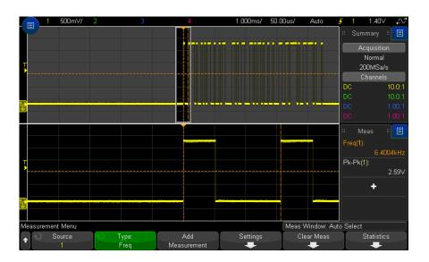
Figure 50 Isolating an event for Frequency measurement
