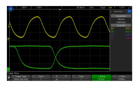
**9** Press the **< Hold** softkey, and turn the Entry knob to select the hold time.
