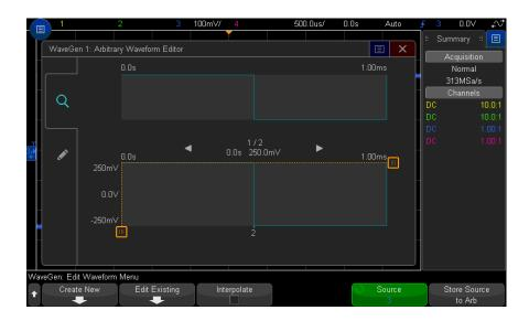
When you open the Edit Waveform Menu, you see the existing arbitrary waveform definition. The voltage and time period you see in the diagram are the bounding parameters — they come from the frequency and amplitude settings in the main Waveform Generator Menu.
