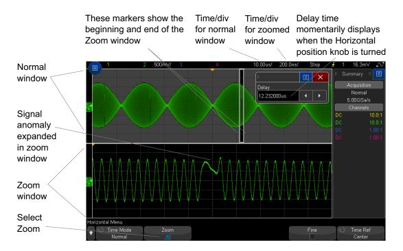
The area of the normal display that is expanded is outlined with a box and the rest of the normal display is ghosted. The box shows the portion of the normal sweep that is expanded in the lower half.
