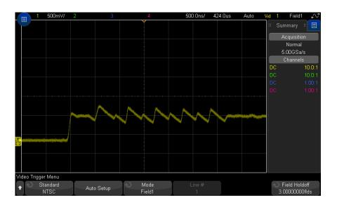
Using Field Holdoff to Synchronize to Color Field 1 or 3 (Field 1 mode) Figure 34
