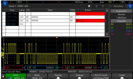
Depending on the selected word decode format, the ARINC 429 decode display is color coded as follows:
