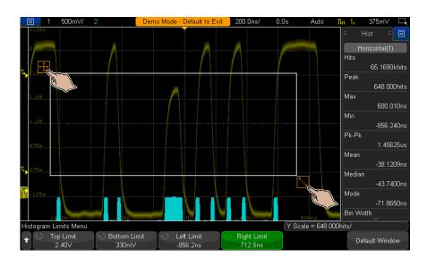
You can also adjust the size and location of the limits window by using the **Top Limit**, **Bottom Limit**, **Left Limit**, or **Right Limit** softkeys and the Entry knob or keypad dialogs.
