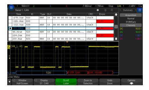
In addition to the standard Time column, the CAN Lister contains these columns:
