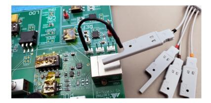
**4** Connect a grabber to one of the probe leads. (Other probe leads are omitted from the figure for clarity.)
