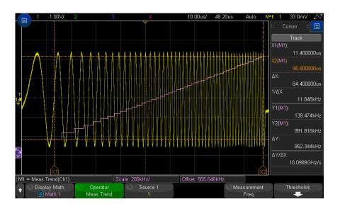
Figure 18 Example of Measurement Trend
