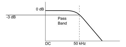
You can use HF Reject to remove high-frequency noise, such as AM or FM broadcast stations or noise from fast system clocks, from the trigger path.
