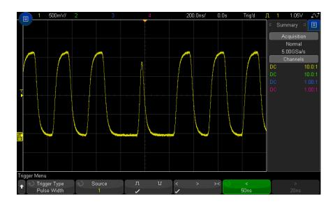
3 Press the **Source** softkey; then, rotate the Entry knob to select a channel source for the trigger.
