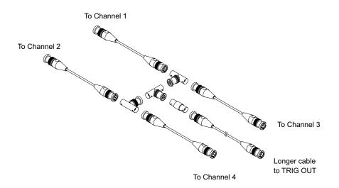
Figure 52 User Calibration cable for 4-channel oscilloscope
