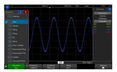
3 Depending on the selected waveform type, use the remaining softkeys and the Entry knob to set the waveform's characteristics.
