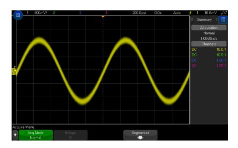
Figure 40 Random noise on the displayed waveform
