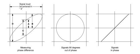
Figure 3 XY time mode signals, centered on display
