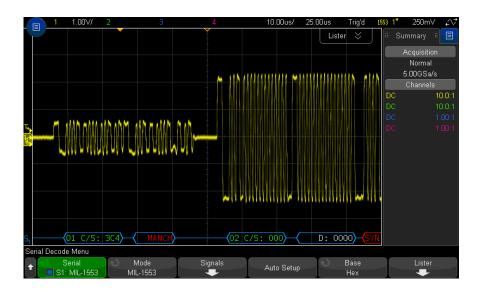
The MIL-STD-1553 decode display is color coded as follows:
