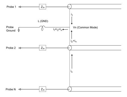
Figure 26 Common Mode Input Voltage Model
