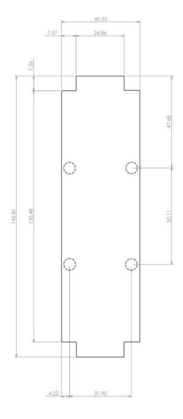
Dashed line shows outline of the mounting boss under PCB board Recommended mounting holes diameter ø3,5mm
