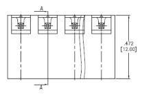
Positions: 02 thru 24  $A = .200 [5.08] \times No. of Positions$   $B = .200 [5.08] \times No. of Spaces$
