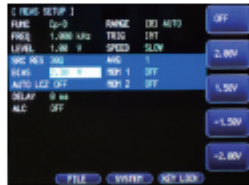
Internal Bias (±2.5V Adjustable) Ideal for Capacitive Components' Characteristic Tests
