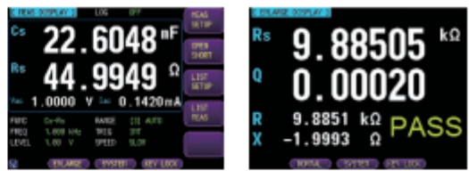
MEAS Display ENLARGE Display Parameter Setting and Four Measurement Parameters Enlarge Measurement Results and Include PASS/FAIL Judgment
