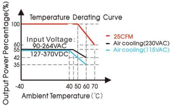
2367913, 2367916 Input Voltage Derating Curve
