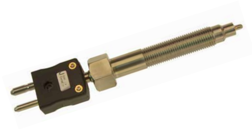
A 1/2"UNF-20 Melt Bolt Thermocouple with Type 'J' Thermocouple Plug
