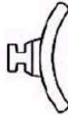
(LFTE) Large Full Trough Element 245 x 60mm (9.6" x 2.36")
