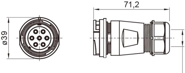
Cable outer diameter range: 13-16mm
