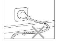
Only use a power supply cable in perfect working order! Do not damage or improperly repair the power cable (tearing, squeezing, running over, ...).
