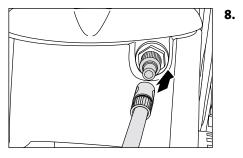
Connect water hose to water inlet (minimum requirements; 5 m hose length, cross-section ¾", 10 bar). The high-pressure cleaner may be connected to a water mains (1-10 bar pre-pressure) with either cold or hot water (up to 60 °C). The medium quadro series provides the opportunity of sucking in water out of a container (see direct suction).
