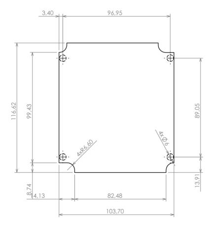
Dashed line shows outline of the mounting boss under PCB board Recommended mounting holes diameter ø3,5mm
