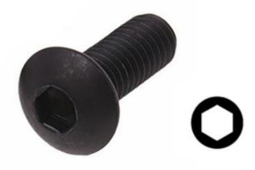
Button Head Socket Screws are designed for light duty. They have a similar thread design as a Socket Cap Screw although the dome shaped head is wider and has a lower profile than a Socket Cap Screw, presenting an aesthetic appearance to an assembly. These fasteners are ideal when a wider bearing surface is required.
