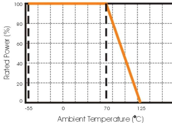
Figure 2 Maximum dissipation in percentage of rated power as a function of the ambient temperature for MCWR12, MCWR08, MCWR06, MCWR04
