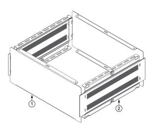
2. Complete Side Frames and Front Rear Panel assembled.
