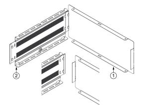
Assemble Side Frame to Front Rear Panel.
