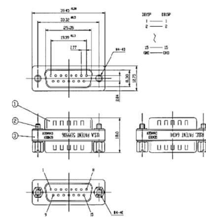
ELECTRICAL : CURRENT RATING 5 Anp Max. CONTACT RESISTANCE 25m? Max. INSULATION RESISTANCE 10000 D Mm. (at 5007 DC: DIELECTRIC WITHSTANDING VOLTAGE
