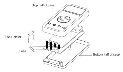
Fuse 0.25A, 5 x 20mm, fast blow, 250V, HBC 1.0KA
