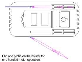
Wrap the leads around the holster to store the test probes.
