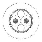
Cable Marking: RS PRO 2 Core×0.5mm<sup>2</sup> Screened Cable 30V
