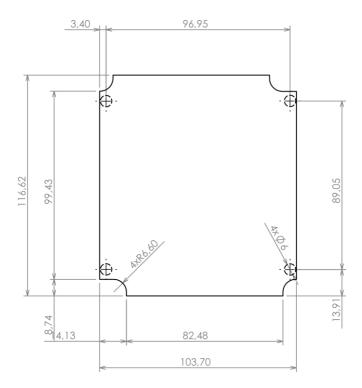
Dashed line shows outline of the mounting boss under PCB board Recommended mounting holes diameter  $\emptyset 3,5 \text{mm}$
