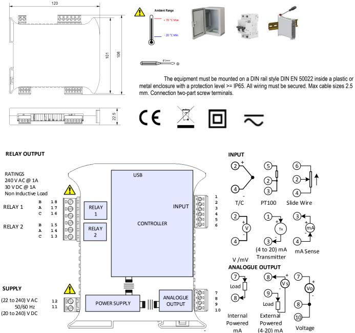
Input connections for cable length >3 metres use screen or twisted pair cables. Thermocouple connections use the correct compensating cable. PT100 connection all wires must be equal length (resistance). Max cable run 30 metres.
