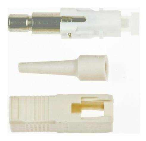
The Optronics SC optical fibre connector is comprised of a polymer body and a ceramic ferrule/spring/crimp barrel assembly plus a crimp over sleeve and rubber boot. These connectors are suitable for, 900µm and 2 and 3mm cables. The connector is precision made and manufactured to demanding specifications. The combination of a ceramic ferrule and a precision polymer housing provides consistent long-term mechanical and optical performance.
