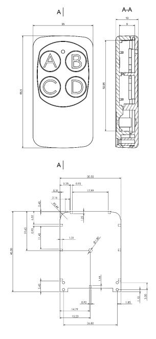
All dimensions are given within +/-0,5mm tolerance
