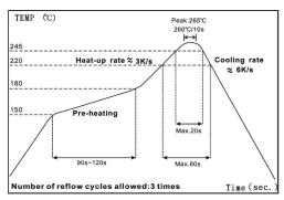
**IR Reflow Soldering**
