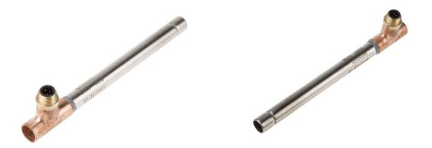
Air heaters feature an open coil of high temperature resistance wire electrically isolated in a stainless steel sheath. Because the air being heated passes directly over the resistance wire, maximum heat transfer efficiency is achieved. Ar heaters are used for heat staking, plastic welding, laminating, drying, heat sealing, and any other operation where air needs to be heated up 500°C
