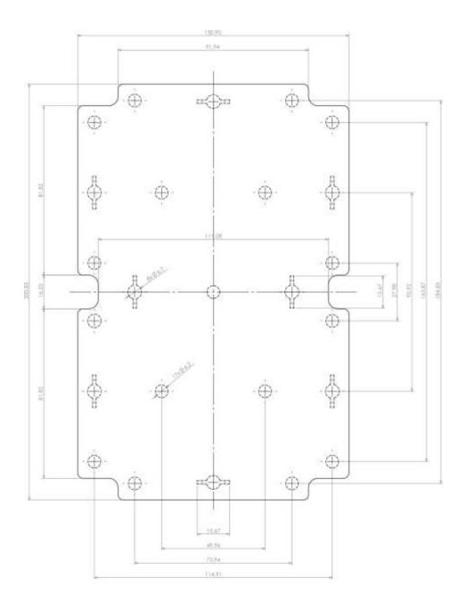
Dashed line shows outline of the mounting boss under PCB board Recommended mounting holes diameter ø4mm
