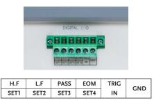
The Digital I/O of IDM-8351 provides two different modes which are general and self-definition. With the general mode, Digital I/O will output Hi Fail, Lo Fail, Pass and EOM (measurement results) based upon the results of the compare function and, furthermore, external trigger input is also provided. Under the selfdefinition mode, users can define output conditions for four pins (SET1~SET4) to execute the external control.
