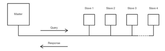
In the MODBUS Protocol the master can address individual slaves, or, using a special "Broadcast" address, can initiate a broadcast message to all slaves. The 236-9298 Digital meter do not support the broadcast address.
