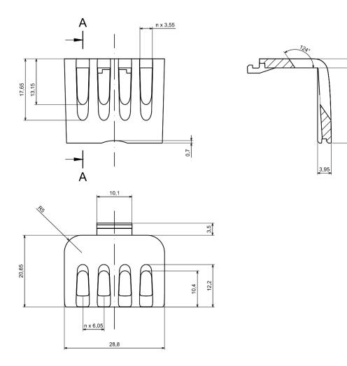
All dimensions are given within +/-0,5mm tolerance
