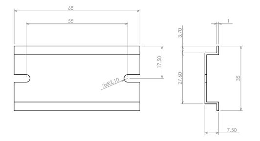
All dimensions are given within +/-0,5mm tolerance
