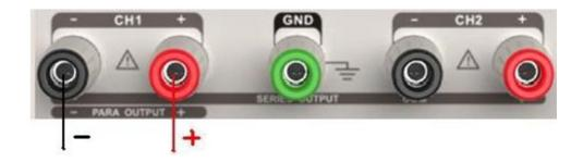
Output ratings  $0\sim30\text{V}/0\sim6\text{A}$  (Max: 32V, 6.4A)
