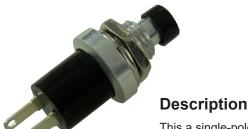
This a single-pole single-throw miniature pushbutton switch with NC contact type, push to break, panel mounting and momentary action.
