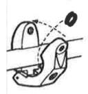
3) Engage screw and tighten until clamp is secure. DO NOT OVER TIGHTEN.
