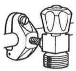
5) Turn clockwise until pipe is penetrated. Set tap to required position.
