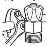
7) The tap is now ready for use. Connect hose to  $\frac{3}{4}$ " BSP thread on tap and turn on. Check for leaks.
