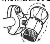
6) Tighten hexagonal nut towards the pipe to secure tap in position.
