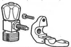
2) Fit the clamp around a clean section of 15mm copper pipe in required position and ensure clamp washer is correctly located.
