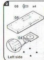
Before assembling. please make sure the position you want to set up (right or left). If you like to set it up in the left side, turn the "L" sign of the slider 04 onward. If you want to set it up in the right side, turn the "R" sign onward. After making sure the direction, secure slider 04 to the underside of slide support 05 with
