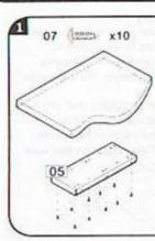
Fit slide support 05 to the underside of your computer desk ensuring it is approximately 15mm back from the front edge, and far enough away from the sides of the desk to enable the CPU to fit under the desk. Using a bradawl mark the screw positions, and secure firmly with screws 07 as shown.
