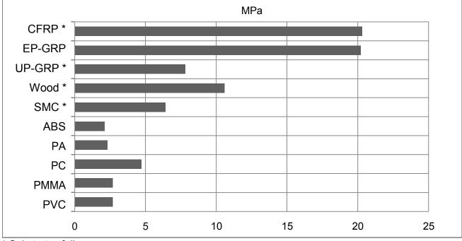
\* Substrates failures
