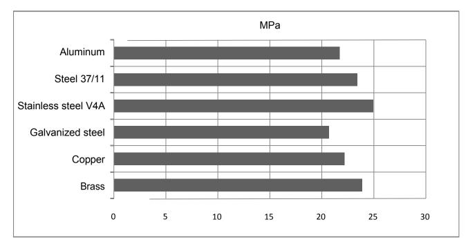
Cured for 16 hours at 104°F (40°C) and tested at 73°F (23°C). Pretreatment - Sandblasting.
