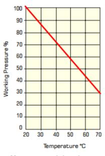
Max. recommended continuous working temperature = 60°C
