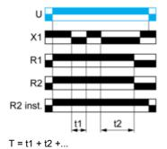
Function: 1 Output with Retrigger / Restart Control
