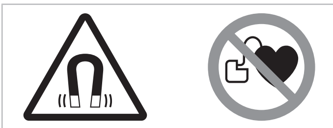
Fig. 15: Warning and prohibition signs on a compressor with LSPM motor
