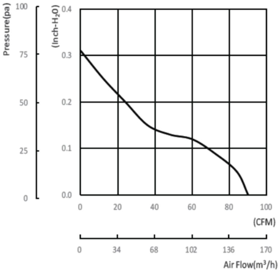
**NOTE:** The airflow and static pressure are measured with specific fixture.
