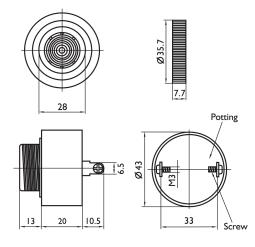
Dimensions : Millimetres Tolerance: ±0.5mm
