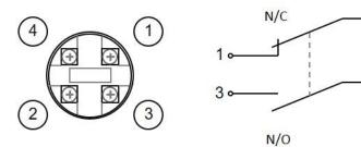
The switch is not polarity sensitive
