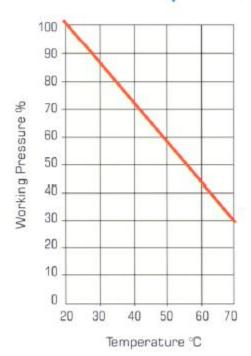
Max. recommended continuous working temperature = 60°C
